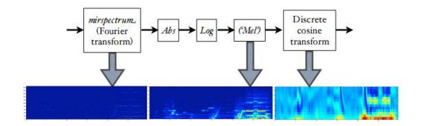
Figure 13: Phases of the MFCC computation (Lartillot, 2008)
