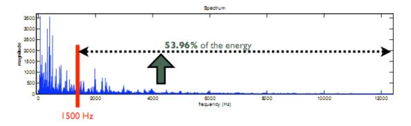
Figure 12: Example of high frequency energy (Lartillot, 2008)
