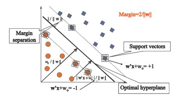
Figure 19: SVM example with optimal separating hyperplane (Ribeiro, 2009)
