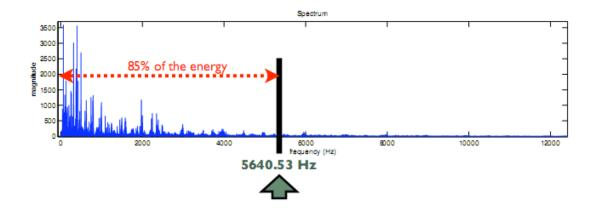
Figure 11: Example of spectral roll off point (Lartillot, 2008)
