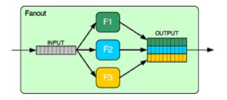
Figure 49: Fanout composite MarSystem
