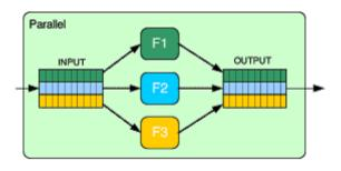
Figure 48: Parallel composite MarSystem
